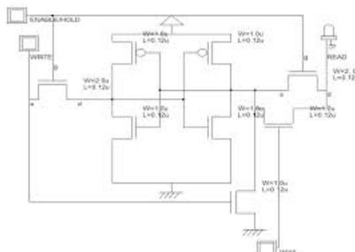
Figure 3: Schmitt Trigger Based SRAM Cell
