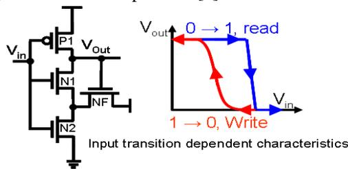
Figure 2: Schmitt Trigger Principle
