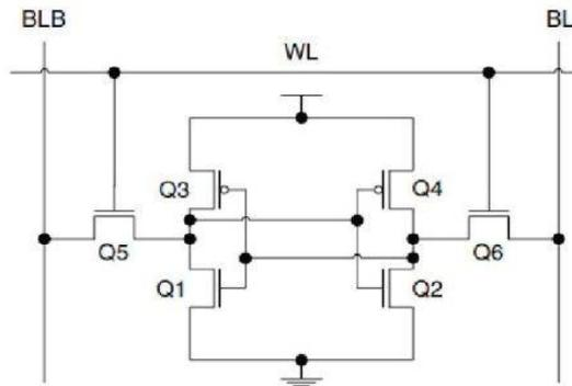
Figure 1: Conventional 6T SRAM Cell
