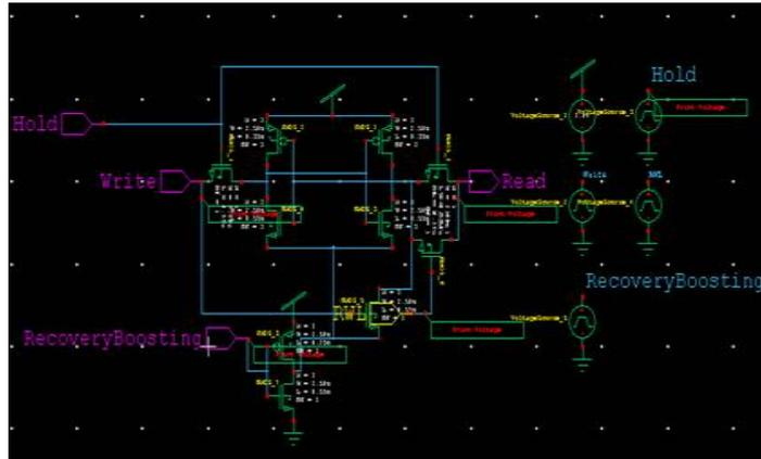
Figure 7: Schematic of SRAM using Recovery Boosting technique
