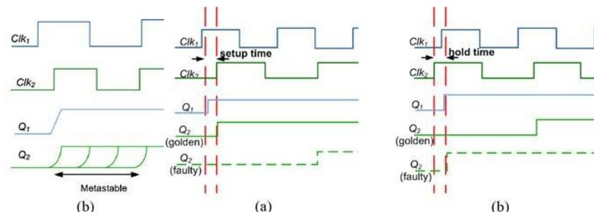
Fig. 1. Example of a CDC circuit and metastability. (a) CDC circuit. (b) Metastability on  $Q_2$
