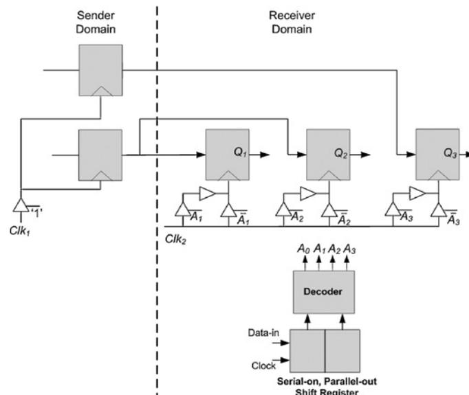
Fig.6 Error recoverable model of the circuit shown in figure 5 with one delay buffer in the clock path of the faulty flip-flop.
