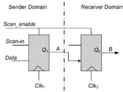
Fig. 3. CDC example for illustrating the proposed ATPG method.
