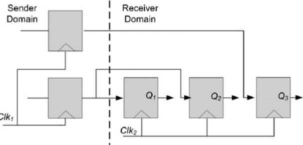
Fig. 4. Example of a CDC circuit (a) with delayed receiver-clock Signal and (b) equipped with an error recovery mechanism.
