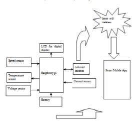
Figure1: Architecture of condition monitoring of wind turbine.
