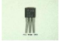
Figure3: Temperature sensor -The LM35.
