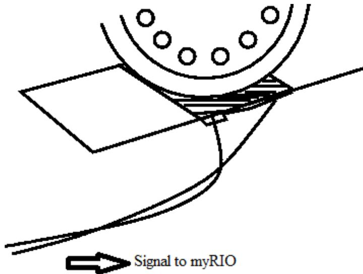
Fig. 4 Load of the Vehicle Acts on Load cell
