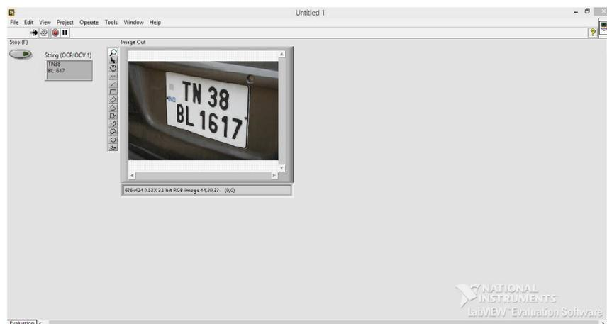
Fig. 9 Number Plate String is obtained
