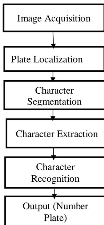
Fig. 8 Block Diagram of Number plate Recognition
