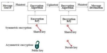
Figure 4: Cryptographic Model
