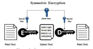
Figure 3 : Symmetric cryptosystems
