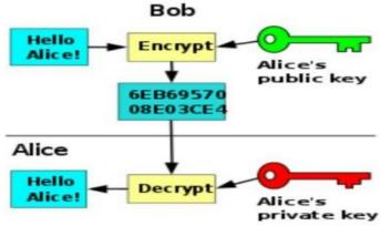
Figure 2: Asymmetric cryptosystems
