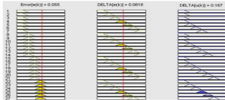
Fig.4.4 Fuzzy rule viewer diagram for fuzzy controller's output, delta [u(k)] Only a portion of rule viewer is shown. Figure 4.5 shows the surf view of fuzzy controller for providing change in duty ratio.
