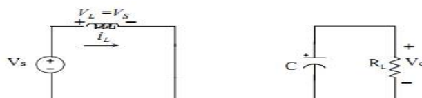
Fig.2.5 Equivalent for DC–DC boost converter during switch ON time
