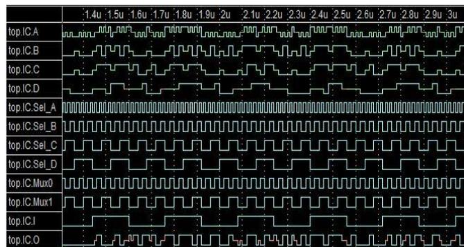
Fig. 8 Waveform of a Connection Block using Verilog-AMS
