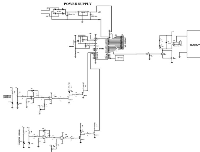
The most cheapest and commonly available energy source of 230v-50Hz and step down, rectifying, filtering and regulating the voltage. A 230v,50Hz single phase AC power supply is given to a step down transformer to get 12V supply.
