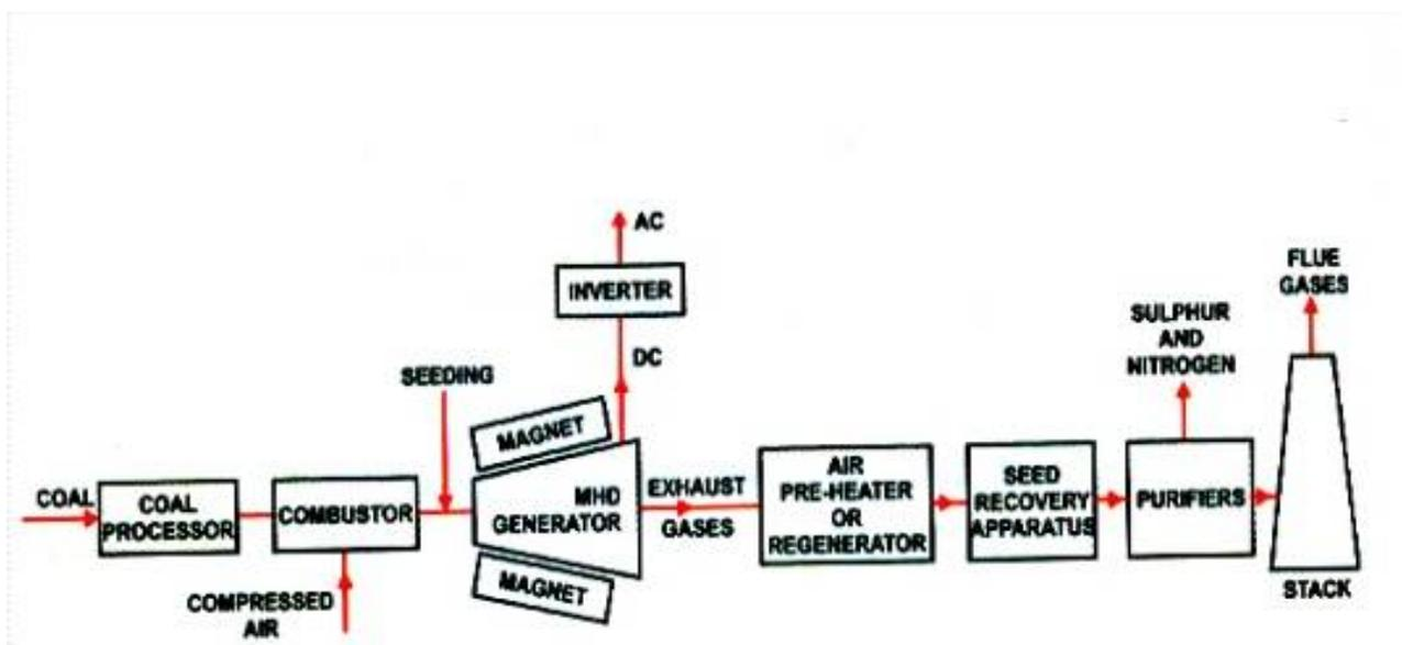
Fig 1. Open Cycle MHD generator
