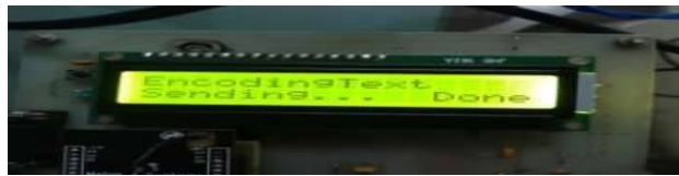
Fig 5.3 Encoding text and sending using zigbee
