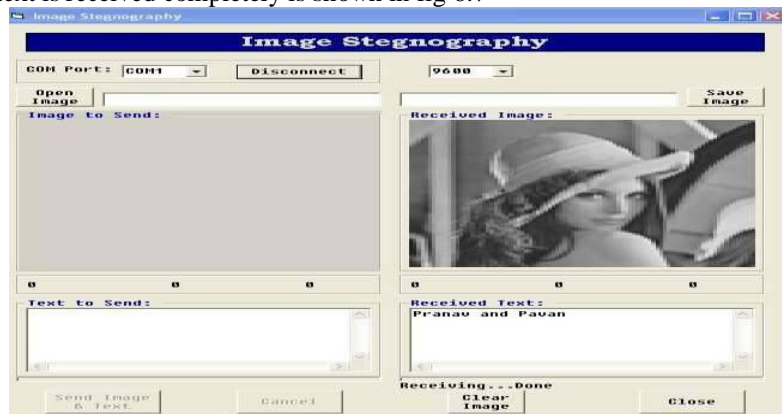
Fig 5.5 Receiving done image and text received successfully
