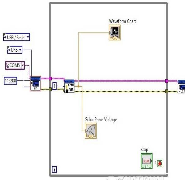
Fig.3 Back panel of LABVIEW
