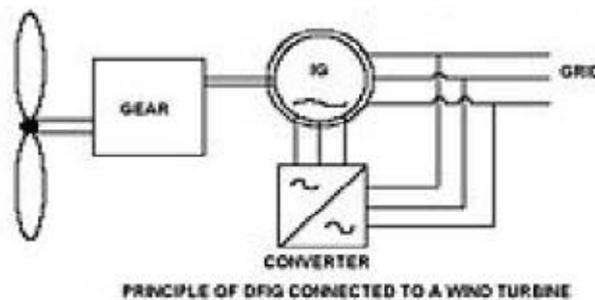
Fig. 4: Principle of DFIG connected to Wind Turbine
