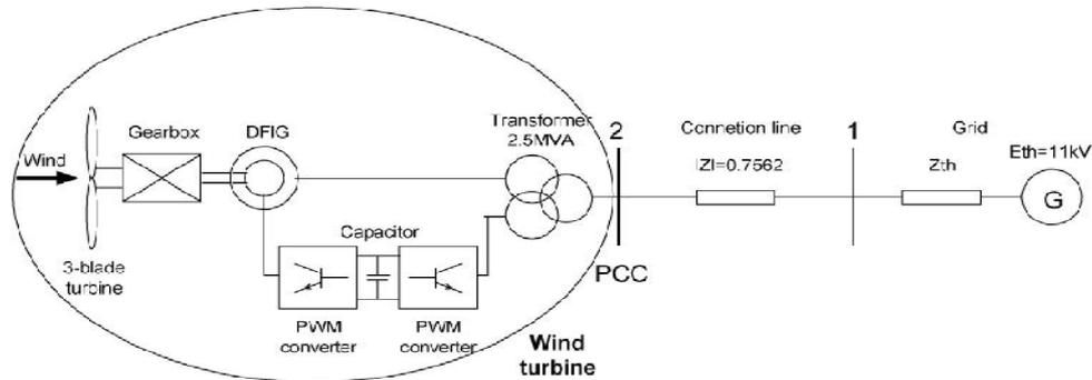
Fig. 3: Overall scheme of the DFIG-based wind turbine system
