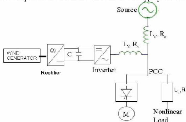
Fig. 5: System with nonlinear load (Thyristor Controlled D.C. Drive)
