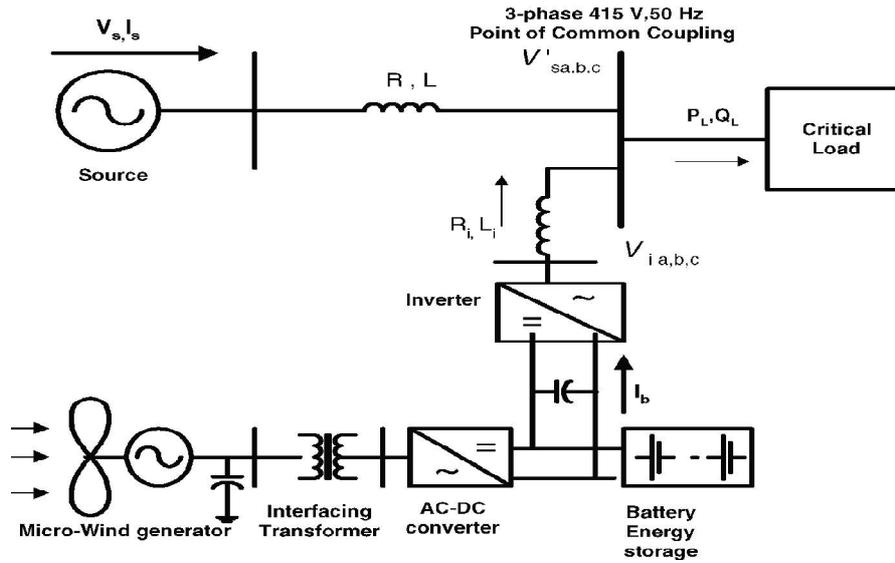
Fig. 6: Scheme of micro-wind generator with battery storage for critical load application.
