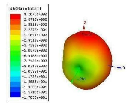
Figure 4 : Gain measurement in dB
