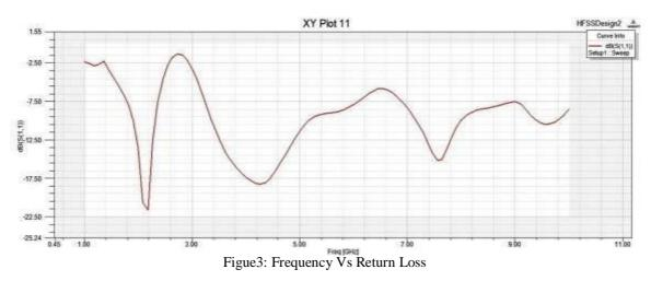
The table3 describes the return loss for the various frequency range in the two different bands. Lower return loss value will increase the performance of the antenna. The maximum gain of the antenna is around 4.2073dB, which is shown in the figure4. The VSWR measurement for this antenna is shown in the figure5, which explains that at which frequency the minimum VSWR is obtained.
