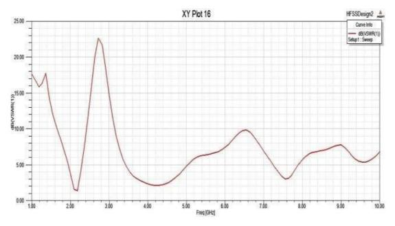
Figue 3: Frequency Vs Return Loss Figure 5: Frequency Vs VSWR
