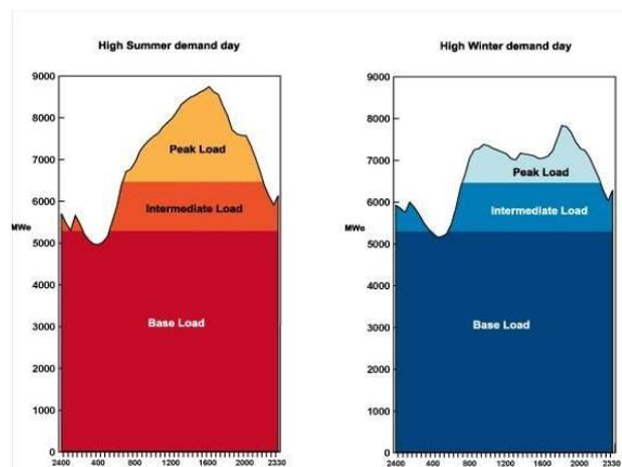
Figure 2: Load curve (courtesy of alfin2300.blogspot.com) [3]
