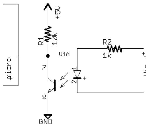
Fig 3 Functional diagram of opto coupler
