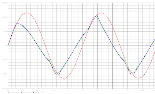
Fig 8 output waveform of chopper with compensative transformer
