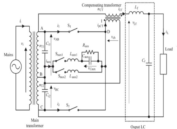
Fig1: Dual-Tap chopping stabilizer with compensating transformer
