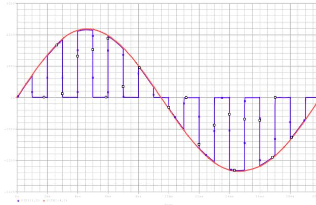
Fig 10 output waveform of dual tap chopping stabilizer with suyclic AC soft switching
