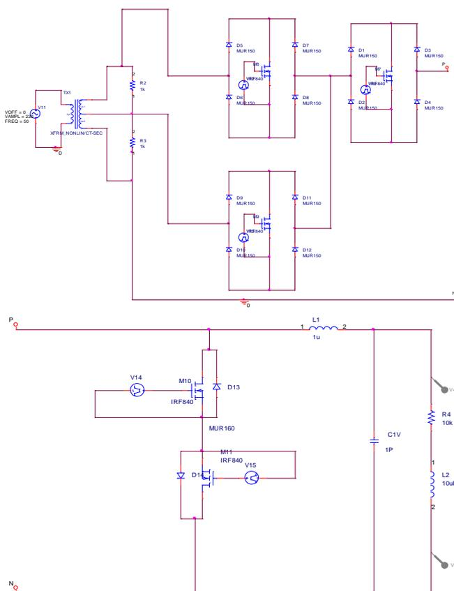
Fig 9: Simulation circuit of dual tap chopping stabilizer
