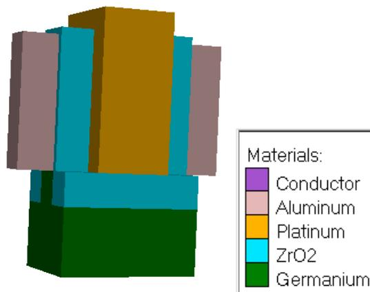
Fig. 5 Trigate FinFET with high-k
