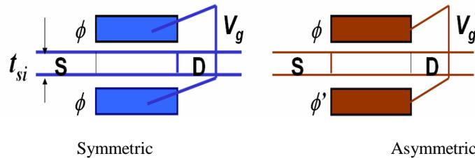
Fig. 2 Symmetric and Asymmetric DG MOSFET[12]
