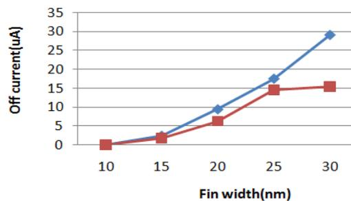
Fig. 1 Off current comparison of DG MOSFET(blue) and TG FinFET(red) as a function of fin width
