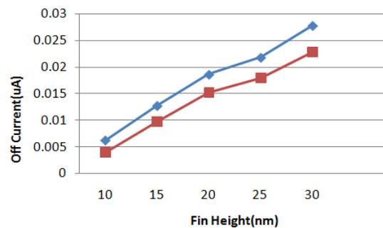
Fig. 2 Off current comparison of DG MOSFET(blue) and TG FinFET(red) as a function of fin height
