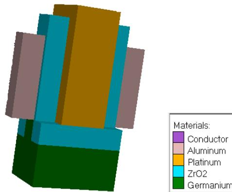
Fig. 4 DG MOSFET with high-k dielectric
