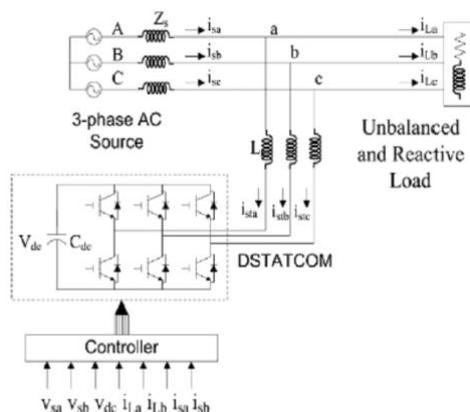
Fig. 1. Basic Circuit Diagram of the DSTATCOM System.
