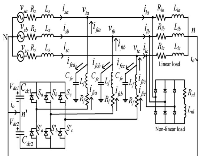
Fig. 2 Circuit diagram of the DSTATCOM-distribution system.
