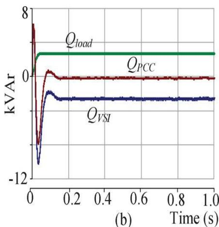
Fig. 6. Load reactive power ( $Q_{load}$ ), compensator reactive power ( $Q_{VSI}$ ), and reactive power at PCC ( $Q_{PCC}$ ). (a) Traditional method. (b) Proposed method
