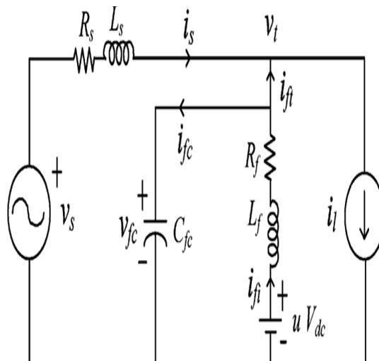
Fig.3 Single-phase equivalent circuit of compensated DSTATCOM.
