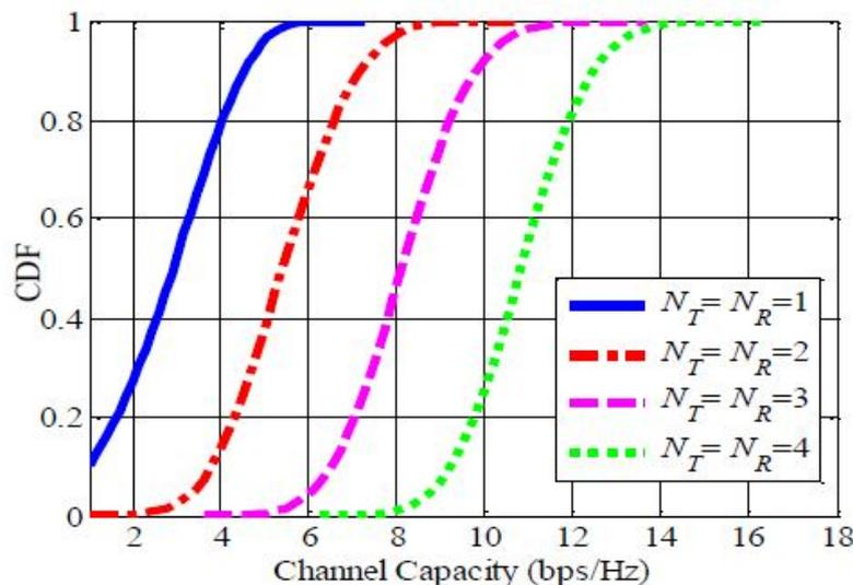
Figure 4. Ergodic MIMO Channel Capacity in Terms of SNR
