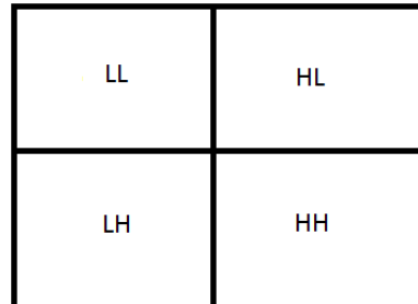
Fig (1): Sub bands obtained from one level decomposition of Image
