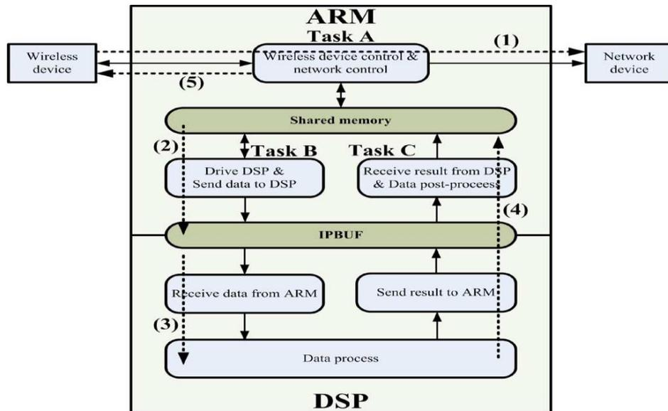
Fig.3. Software structure of the embedded system and the data processing flow.
