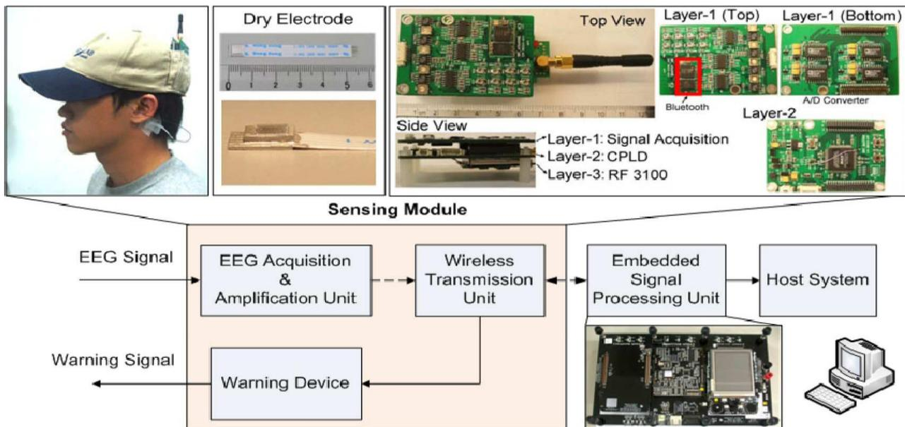
Fig1. Block diagram of the proposed BCI system.
