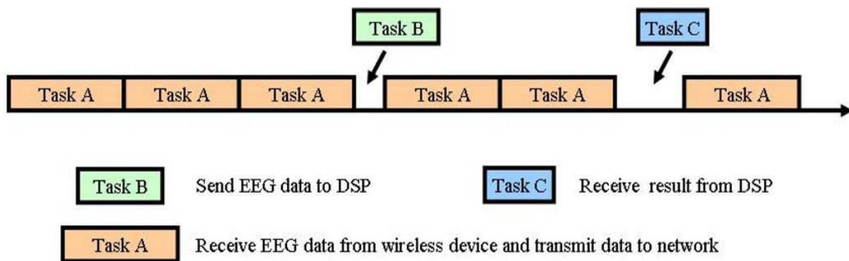
Fig..4. Time series diagram of multitask scheduling mechanism
