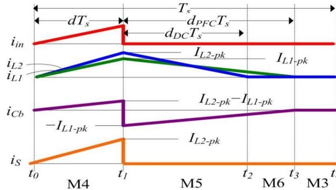
Fig.6 The key waveforms of the proposed S4 converter in region II
