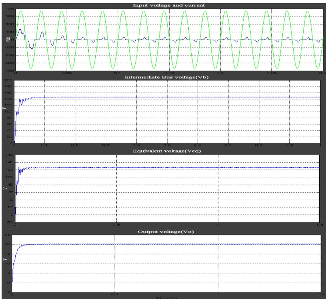
Fig.8 The ISSSDB waveforms of (a) Input voltage and current (c) Intermediate bus voltage (d) Output voltage for input voltage 260 Vrms
