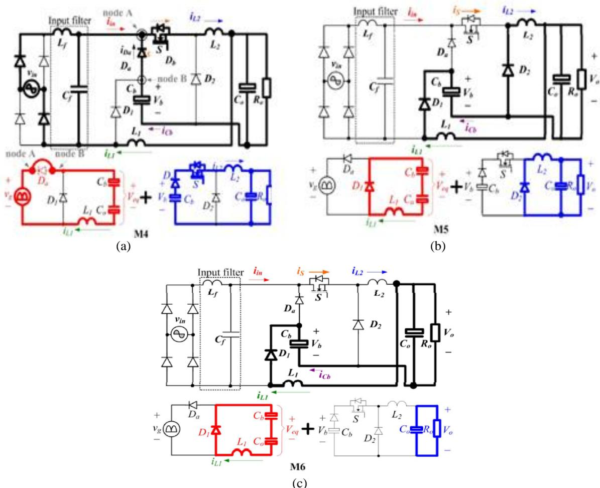
Fig.5 Circuit operation stages of region II of proposed converter
