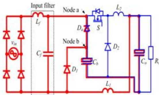
Fig.1 Integrated single-stage single-switch double buck converter
