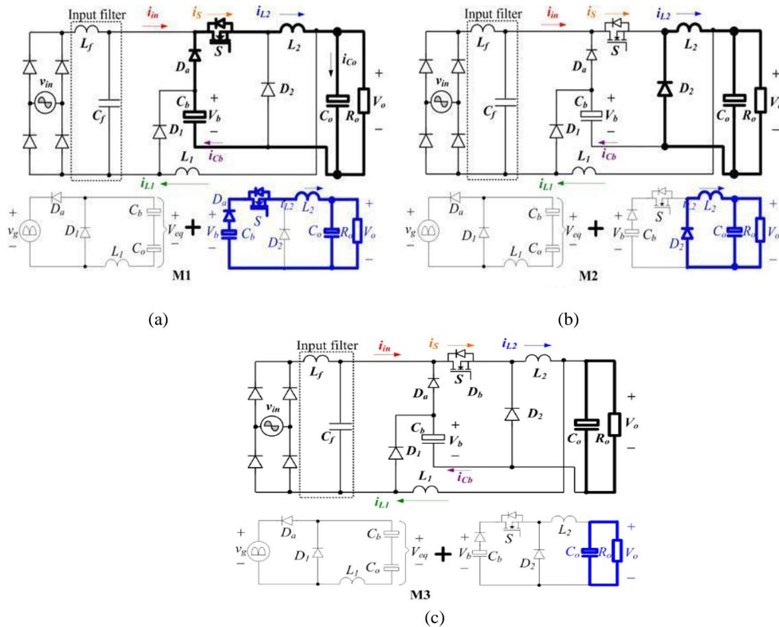
Fig.3 Circuit operation stages of region I of proposed converter
