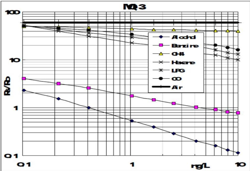
Fig.7 Typical sensitivity characteristics of the MQ-3 for different gases.
