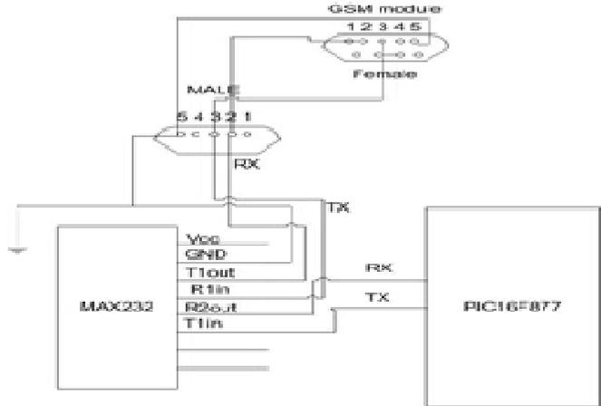
Fig.2 – GSM interfacing
