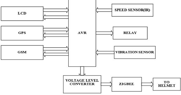
Fig.3 – Block diagram explanation of Bike section
