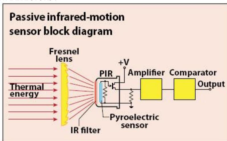
Fig 4: PIR Based Motion Detectors
