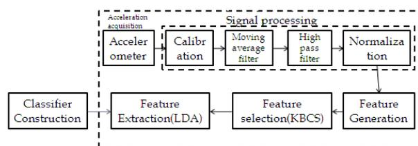
Fig 6: Algorithm Block Diagram
