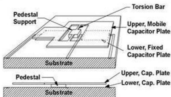
Fig no 2:MEMS Fabrication
