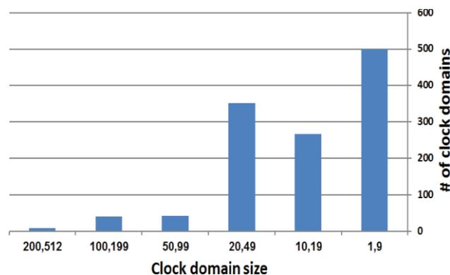
Fig.3. Distribution of the number of FFs sharing a common pre-enabled clock signal of a DSP core
