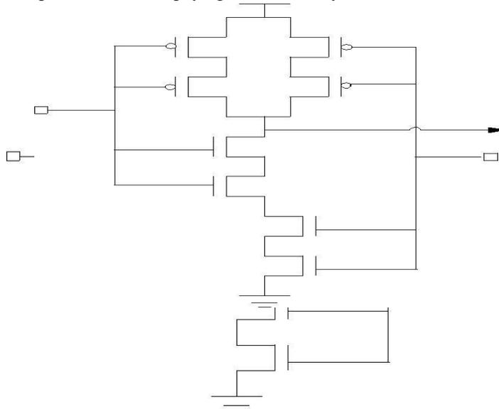
Fig.5.Stack Approach based 2 input NAND gate
