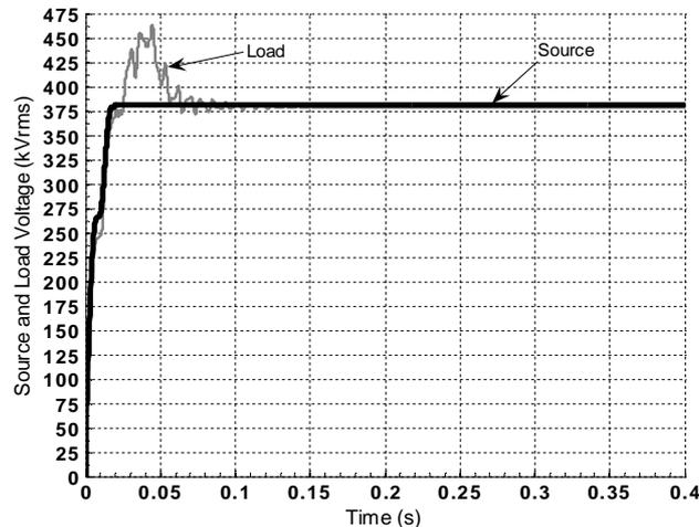
Fig. 6-a. Source and Load Voltage for the system with TSC (Capacitor is not precharged)
