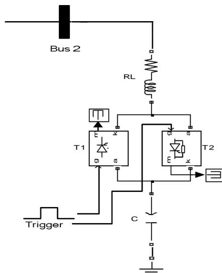
Fig. 2. A single phase TSC configuration
