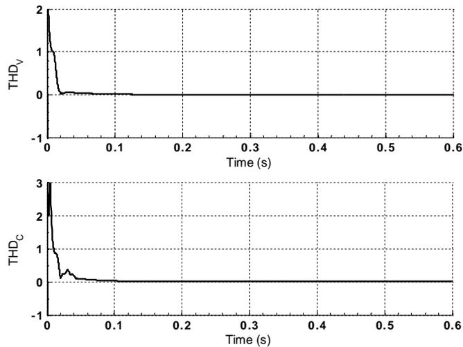
Fig. 10.  $THD_V$  and  $THD_C$  (Capacitor is precharged)
