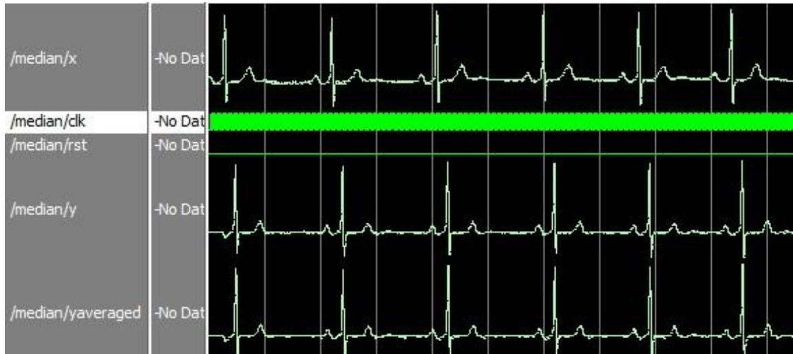
Fig. 5: Waveform for traditional median filter based system (analog mode)
