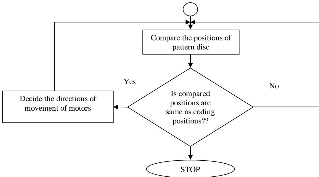
Fig.4: Working flow of Patterned Disc
