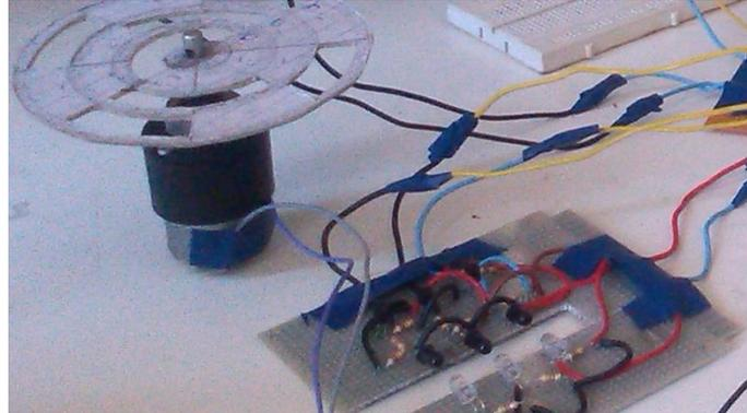
**Fig.3:** Encoder Circuitry
