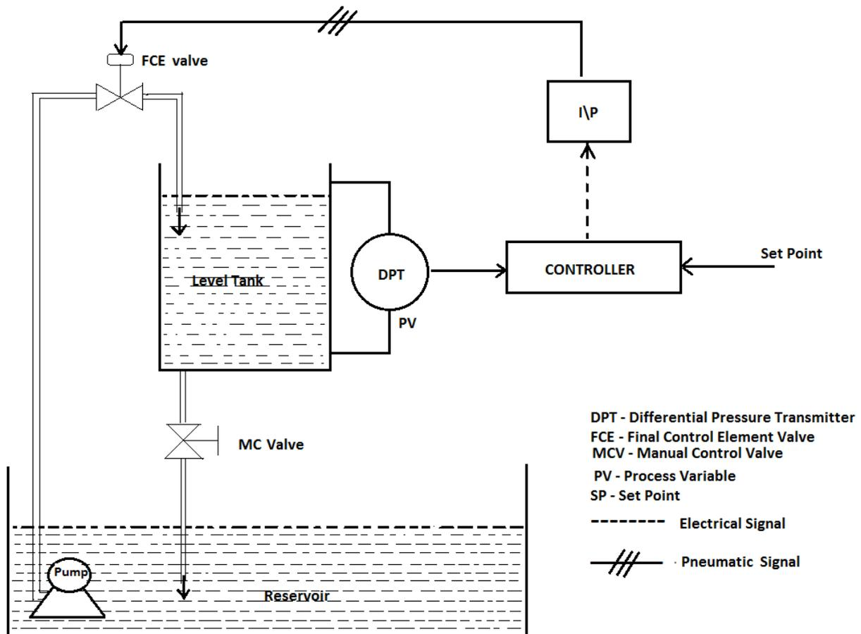
**Figure II.A: Piping and Instruments to Implement the Circuit Diagram**
