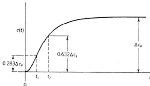
**Figure IV.C: process reaction curve**
