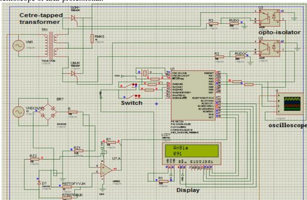
Figure.2 Microcontroller PIC16F72 based triggering circuit on Proteus software ISIS professional editing window
