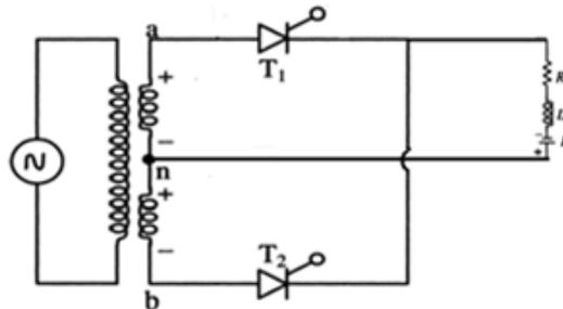
Figure.1 Single phase full wave centre-point converter
