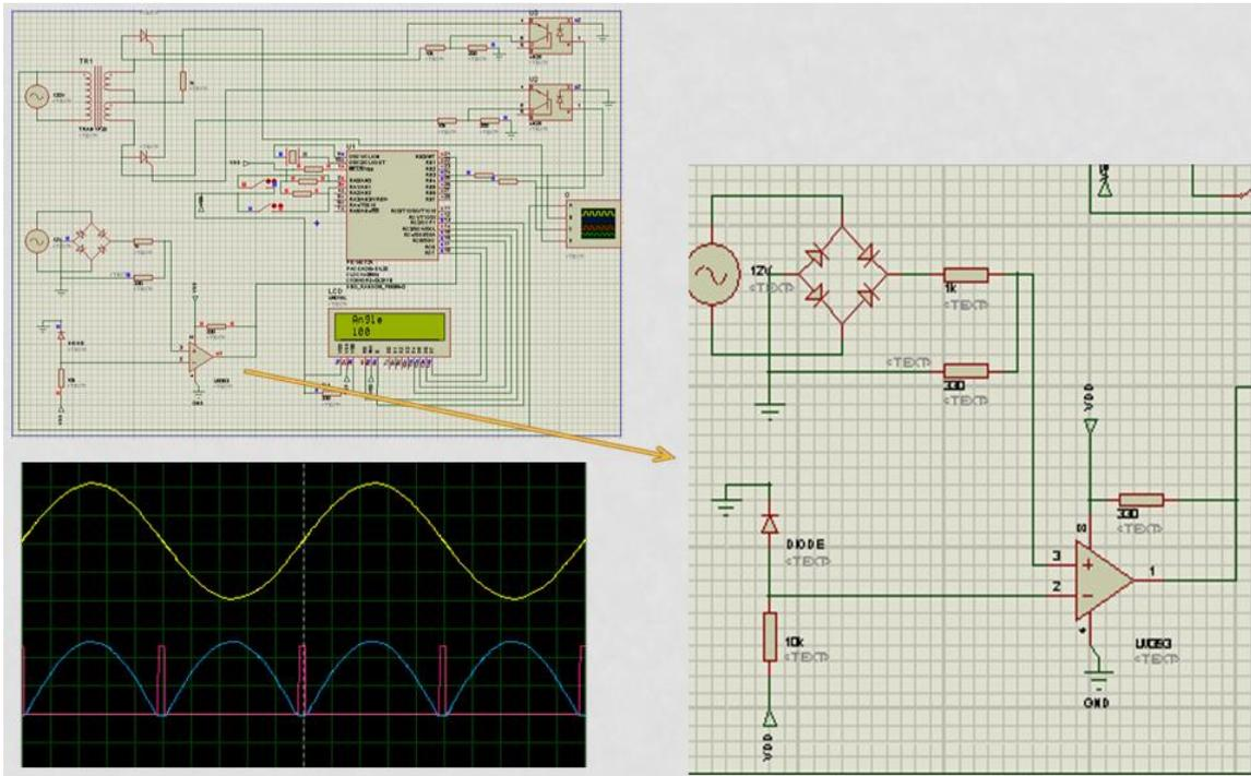
Figure.3 Supply, zero-crossing circuit and synchronised output waveform
