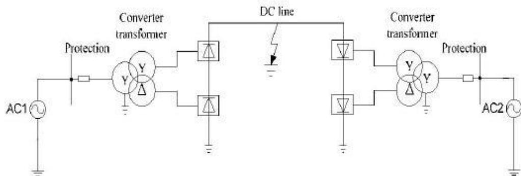
Fig1:Schematic Diagram of HVDC System
