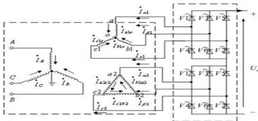
Fig 2: Converter Transformer
