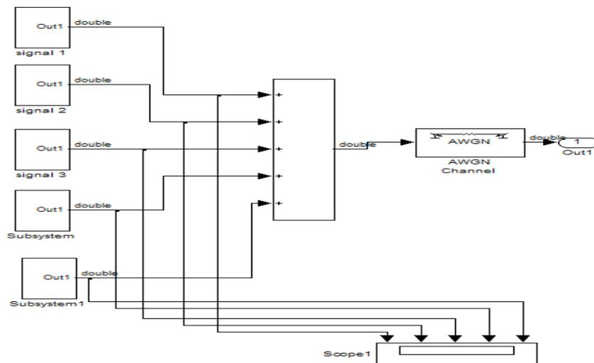
Fig 1(a) Detection of Primary Users using Binary Number series
