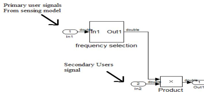
Fig 5(a) Frequency selection for PUs and SUs
