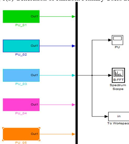
Fig 2(a) Detection of Primary Users Using Bernoulli Random Number Series
