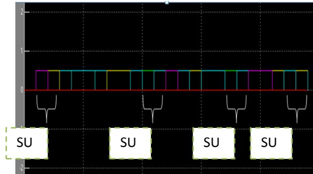
Fig 5(b) Spectrum allocation for PUs and SUs for Binary Number Series
