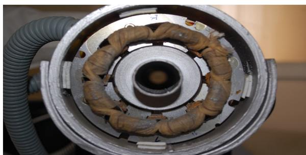
Fig.5. Physical arrangement of Active Magnetic Bearing.
