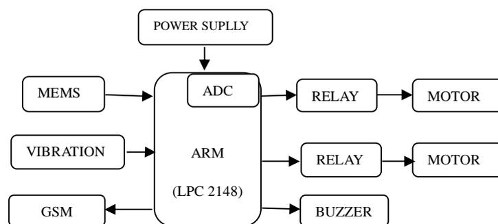
Fig.1 Block diagram of monitoring system in a buildings
