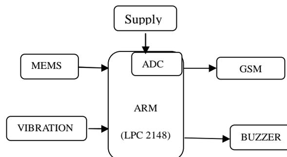
Fig.4 Block diagram of transmitter section
