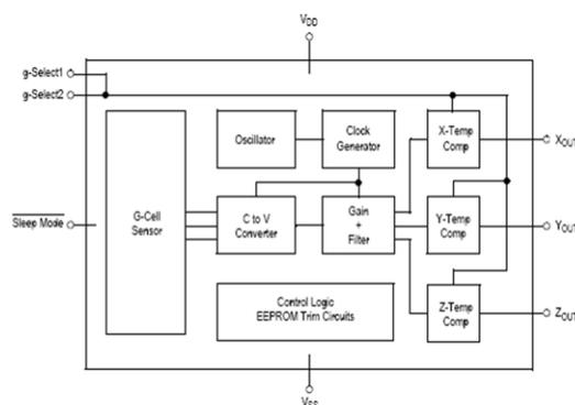
Fig.2 MEMS Block diagram
