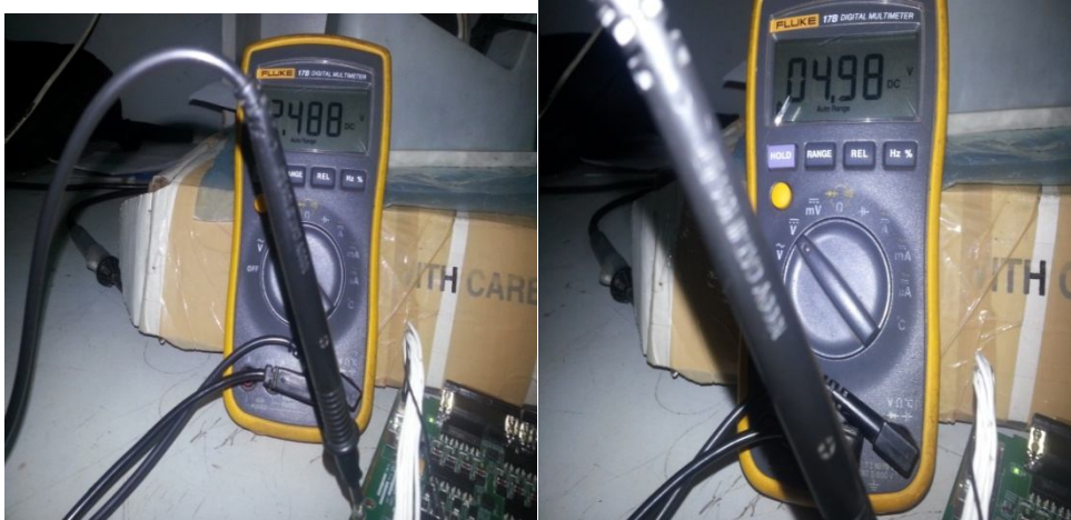
Figure 4.4: DAC output for controlling drive speed
