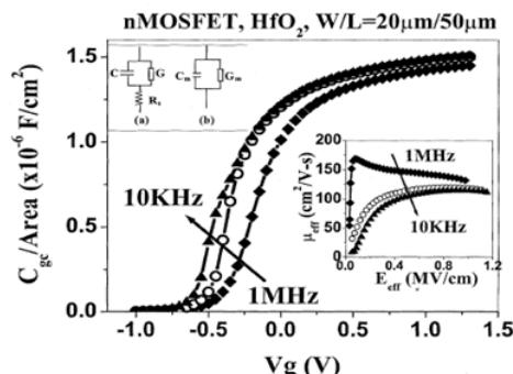
Figure 9: Gate-to-channel capacitances of  $\text{HfO}_2$ -gated n-MOSFET with  $L = 50\mu\text{m}$  measured at three different frequencies. The upper inset shows (a) the equivalent circuit model of the MIS capacitor and (b) the model for parallel capacitance measurement. The lower inset shows the apparent mobility values of this device as extracted from this set of split-C–V curves.
