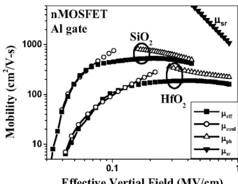
Figure 3: Effective mobility for the two samples,  $\text{HfO}_2$  and  $\text{SiO}_2$  samples due to Coulomb scattering and Phonon scattering
