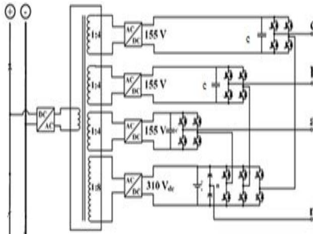
Fig no.1 Proposed cascaded Hybrid Multilevel inverter
