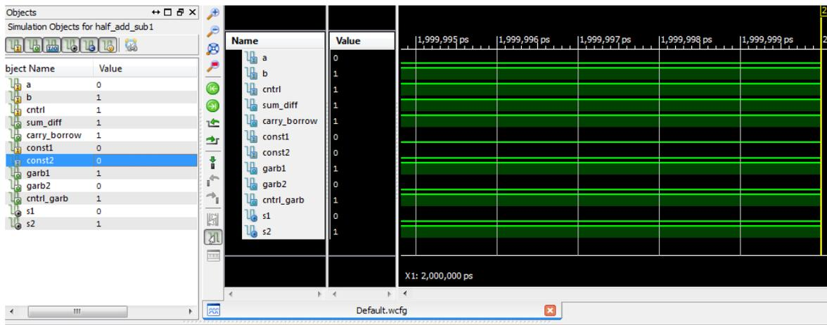
Fig. 13b Simulation result of reversible Half Adder/Subtractor when ctrl=1 (acts as Half Subtractor)
