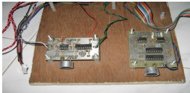
Fig.3. Ultrasonic Transmitter-Receiver Module
