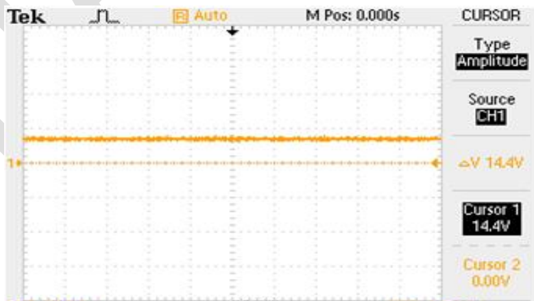
Figure 9 : DC output of Boost Converter
