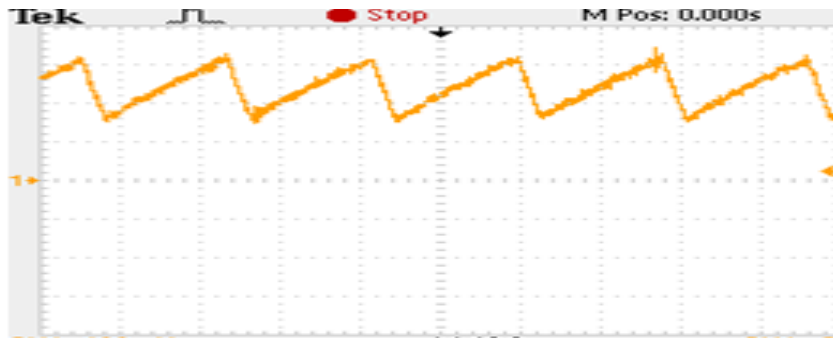
Figure 7: Inductor current of Boost in continuous conduction mode.
