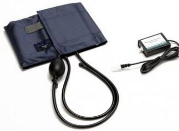
FIG 5: Oscillometric Pressure sensor.
