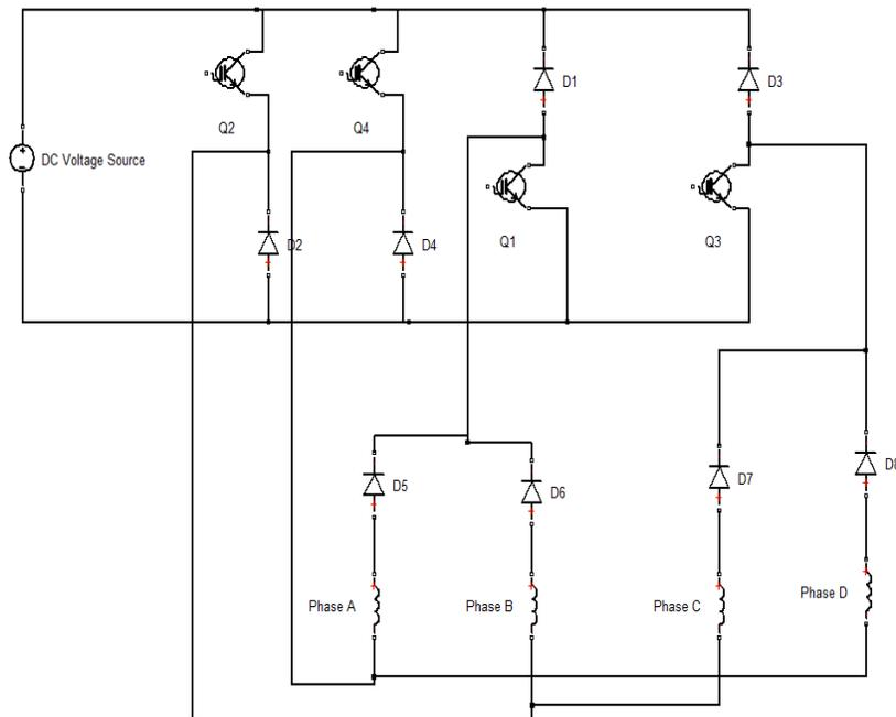
Fig. 4. Modified single-switch-per-phase converter
