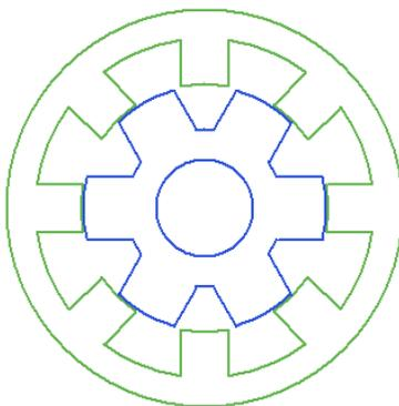
Fig. 2. Switched reluctance machine with four phase and 8/6 poles on both stator and rotor.
