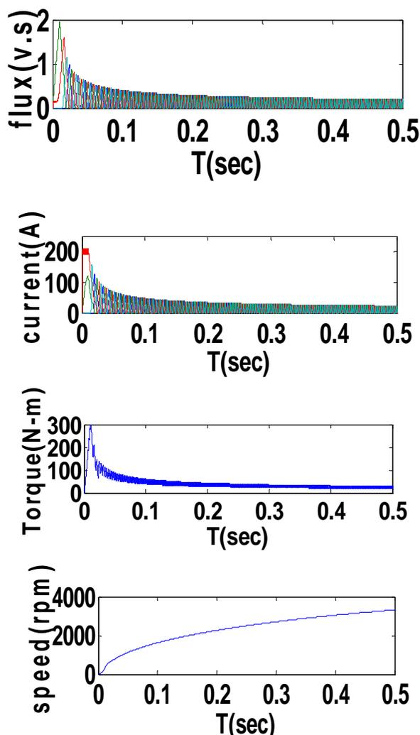
Fig. 14.. Performance characteristics of proposed converter for SRM drive
