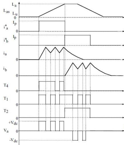
Fig. 8. for overlapping current conduction
