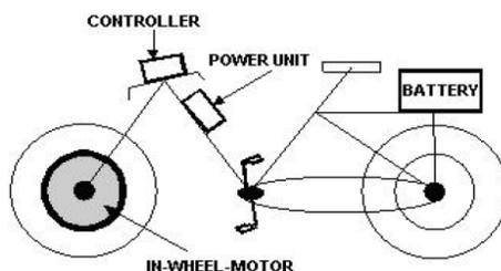
Fig. 1. Structure of the electric bike
