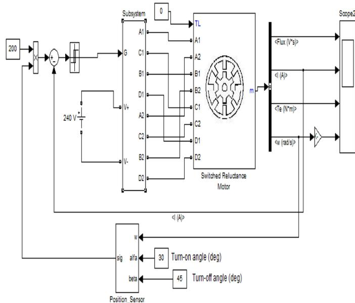
Fig. 12. Complete block diagram of SRM drives
