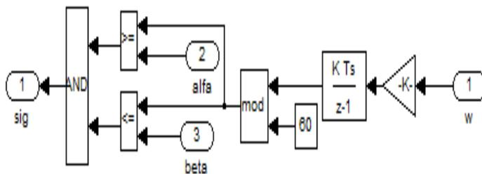
Fig. 13. Position sensor blocks
