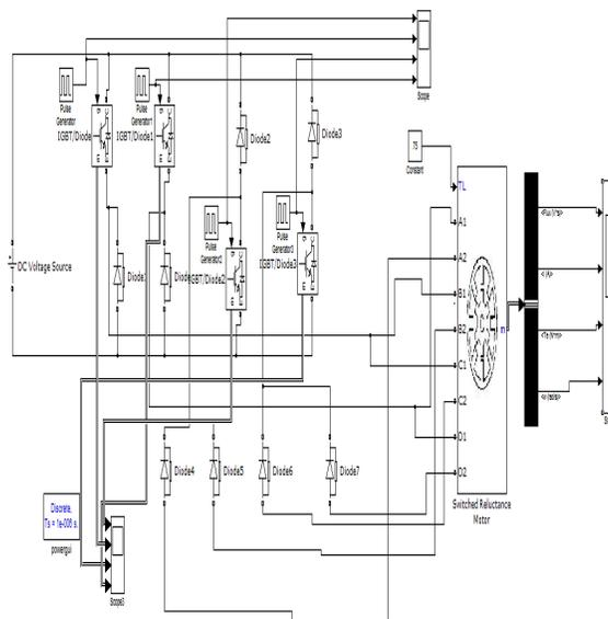
Fig. 9. Proposed Converter with SRM model
