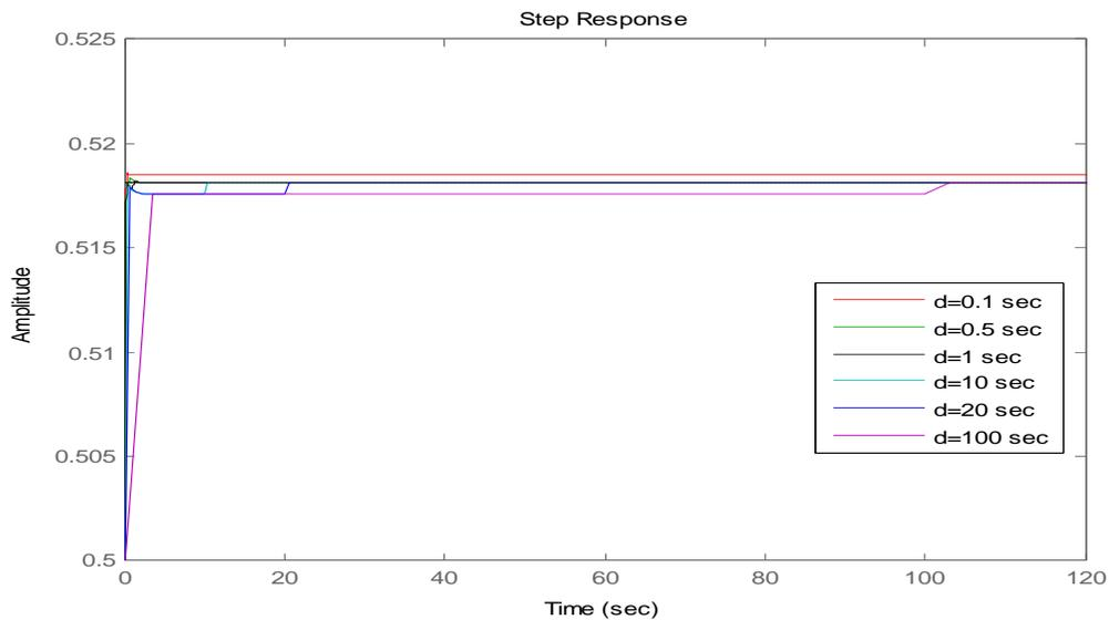
Fig 5 Closed loop responses of the uncertain system with disturbance attenuation bound  $\gamma = 0.5$
