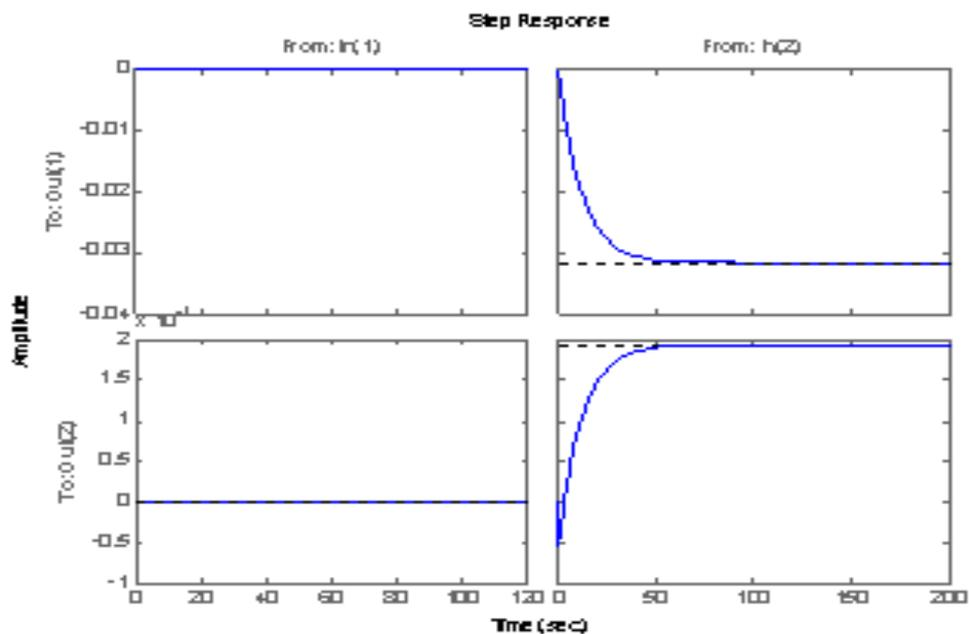
Fig 3 Closed loop response of the system with delay 0.1 sec
