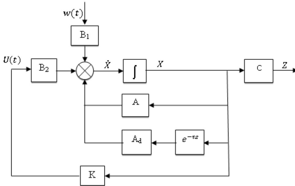
Fig 1. Control scheme for a linear varying time delay system represented by Eqn (1)
