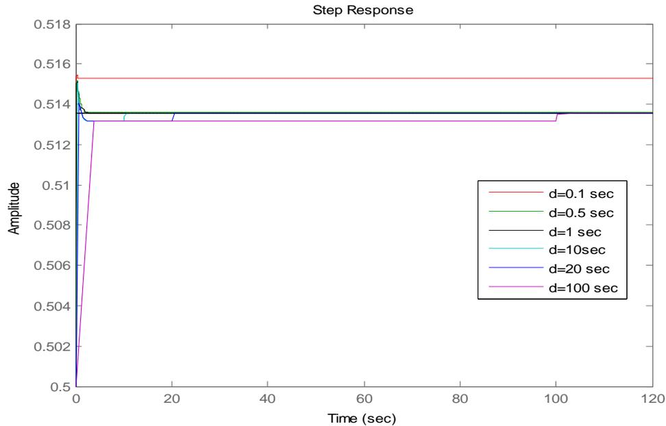
Fig 4 Closed loop responses of the uncertain system with disturbance attenuation bound  $\gamma = 1$
