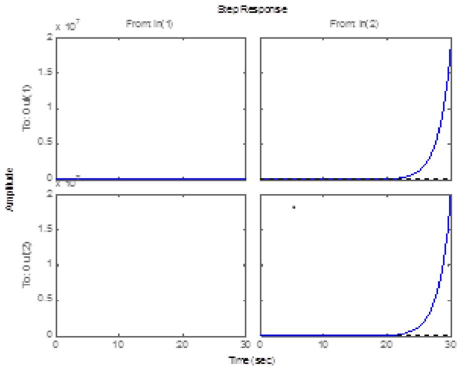
Fig 2 Open loop response of the system with delay 0.1 sec
