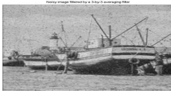
Fig 4: Noisy Image Filtered By A 3 By 3 Averaging Filter
