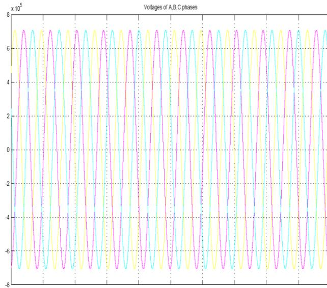
Fig. 10: Voltage waveforms with TCSC in capacitive mode of operation
