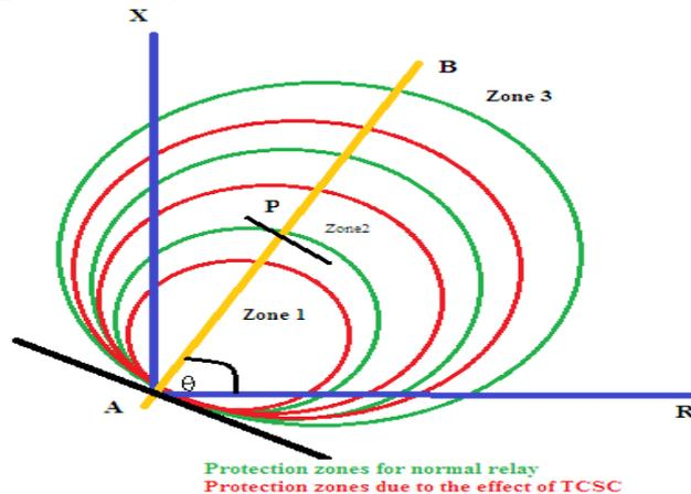
Fig. 6: Combination of Zones of Protection for normal relay and TCSC operation
