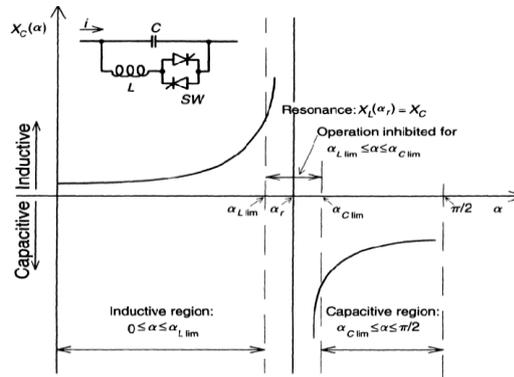
Fig. 2: TCSC reactance versus delay angle  $\alpha$
