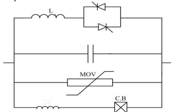
Fig. 1: TCSC circuit configuration
