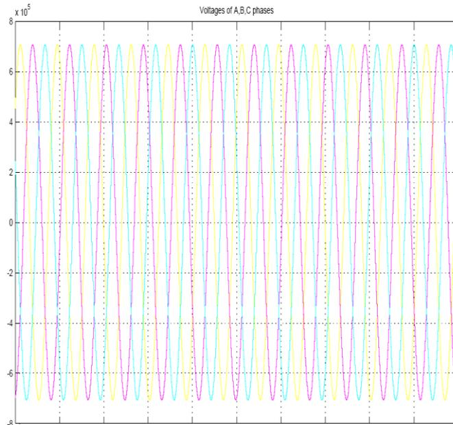
Fig. 8: Voltage waveforms without TCSC
