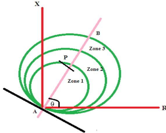
Fig. 4: Typical 3 zones of distance protection relay
