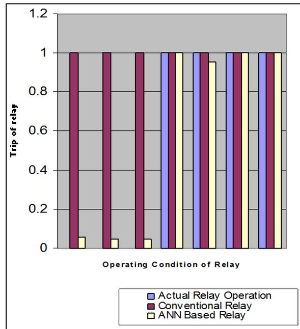
Fig. 12: Bar Graph showing Comparison of Output of Conventional Relay Output with ANN output
