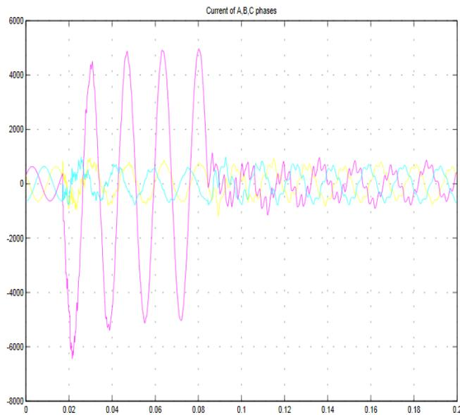
Fig. 11: Current waveforms with TCSC in capacitive mode of operation
