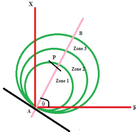
Fig. 5: Zones of protection of a transmission line with TCSC
