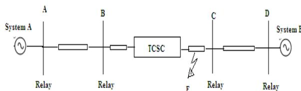
Fig.: 7 Single-line diagram of the test system
