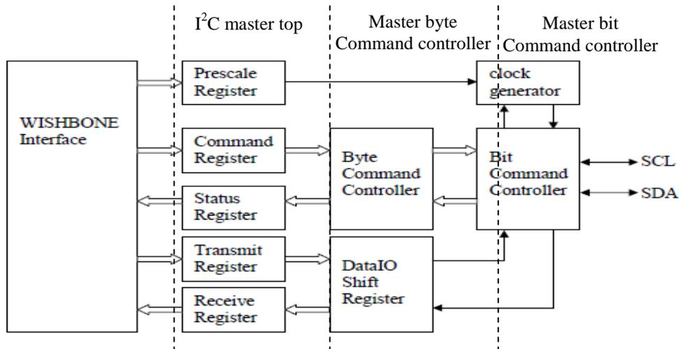
Fig 3: Components in I<sup>2</sup>C communication
