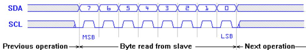
Fig 6: Reception of a byte from a slave
