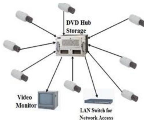
Fig 4: Data Surveillance System
