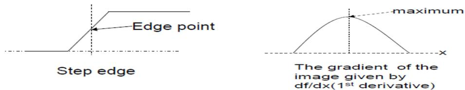
Fig1: Gradient method for Edge detection
