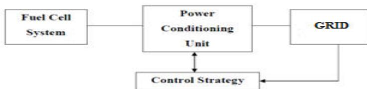
Fig. 6: Block diagram of power conditioning system
