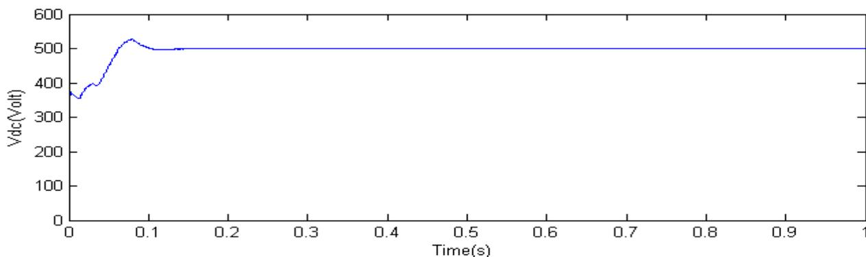
Fig. 8: Output voltage of fuel cell fed boost converter
