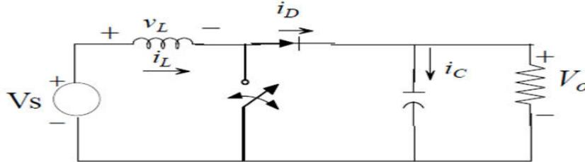
Fig. 2: DC – DC Converter Model
