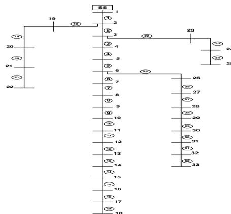
Fig. 2. IEEE 33-node radial distribution system
