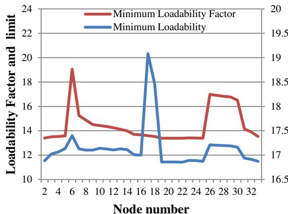
Fig. 6. Variation in minimum loadability factor and limit with capacitor placement at each node.
