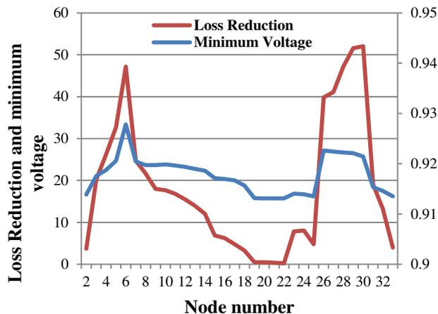
Fig. 5. Variation in loss reduction and minimum voltage profile with capacitor placement at each node.
