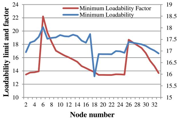
Fig. 4. Variation in minimum loadability factor and limit with DG placement at each node.
