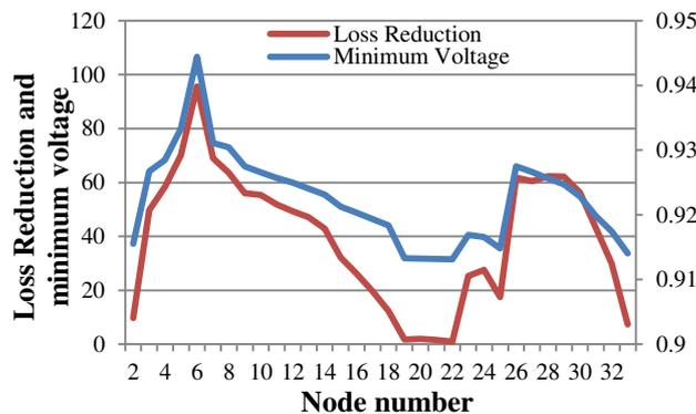
Fig. 3. Variation in loss reduction and minimum voltage profile with DG placement at each node.
