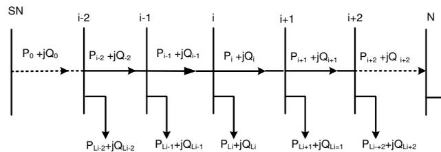
Fig. 1. Single Line Representation of Radial Distribution System.
