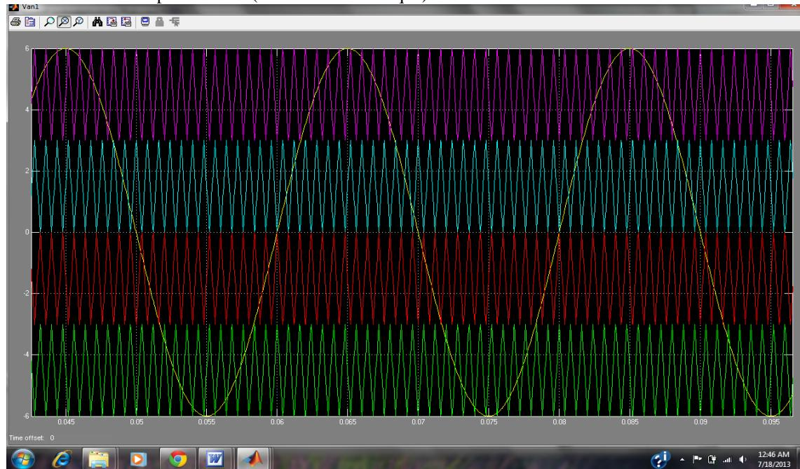
Fig.5 Sine Waveform Simulation of Five Level Diode Clamped Inverter.(POD PWM Technique)
