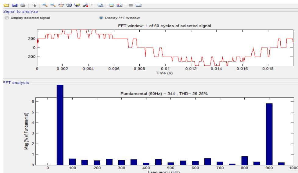
Fig.12 Harmonic Spectrum of Five level diode clamped Inverter Phase Voltage at modulation Index=1 (APOS PWM Technique).
