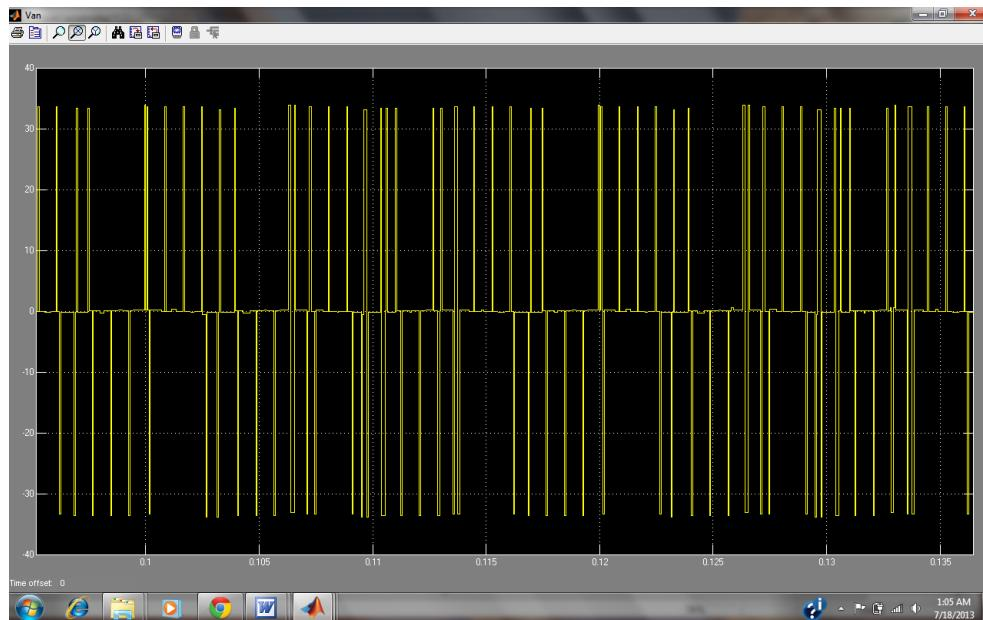
Fig.11 CMV of Five Level Diode Clamped Inverter (APOS PWM Technique)
