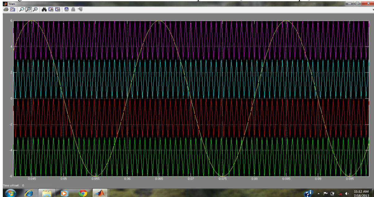
Fig. 1 Sine Waveform Simulation of Five Level Diode Clamped Inverter.(PD PWM Technique)
