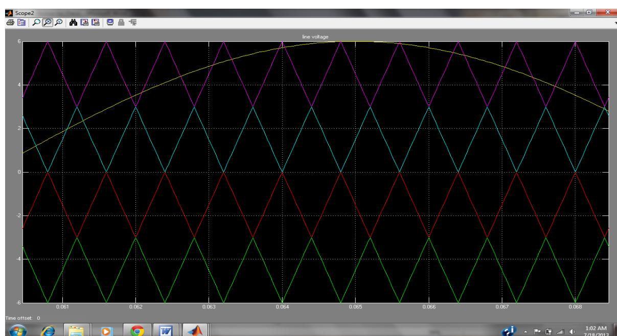
Fig 10 Triangular Waveform Simulation of Five Level Diode Clamped Inverter (APOS PWM Technique)
