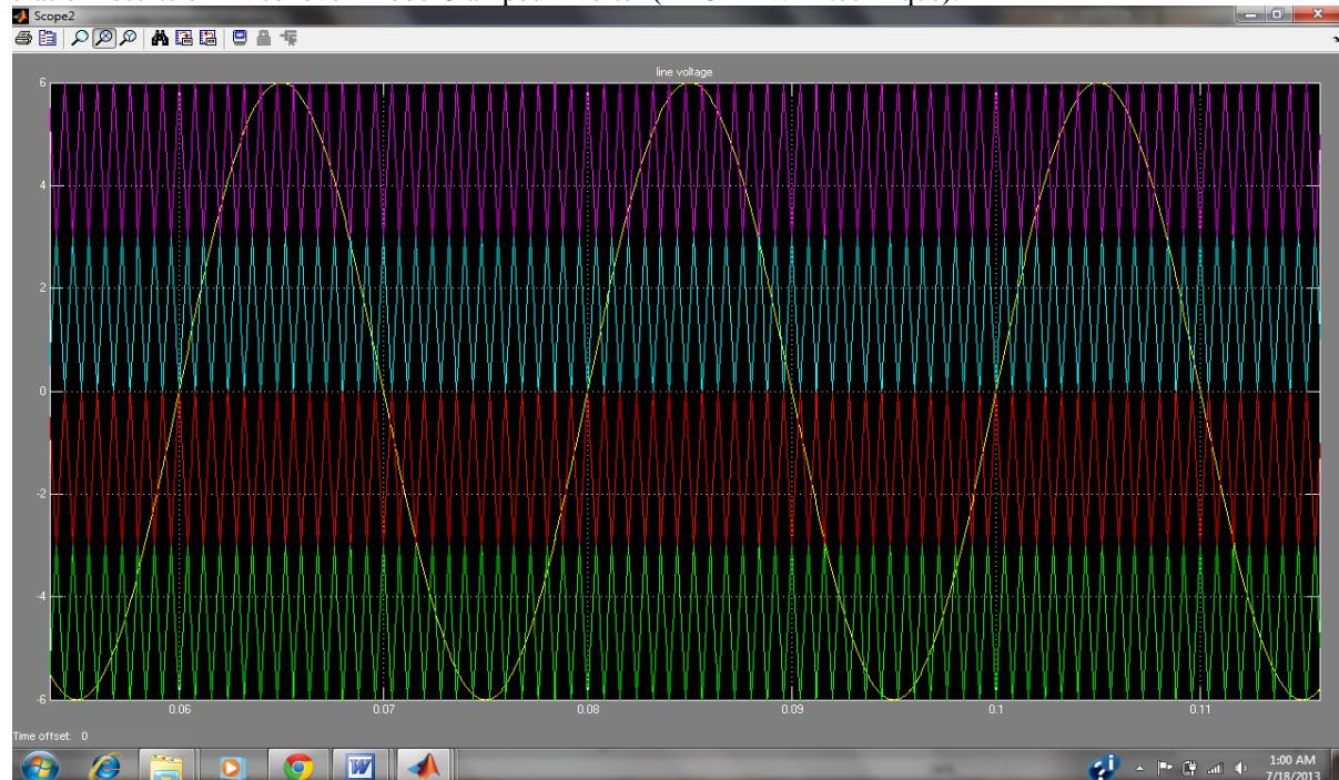
Fig.9 Sine Waveform Simulation of Five Level Diode Clamped Inverter.(APOS PWM Technique)
