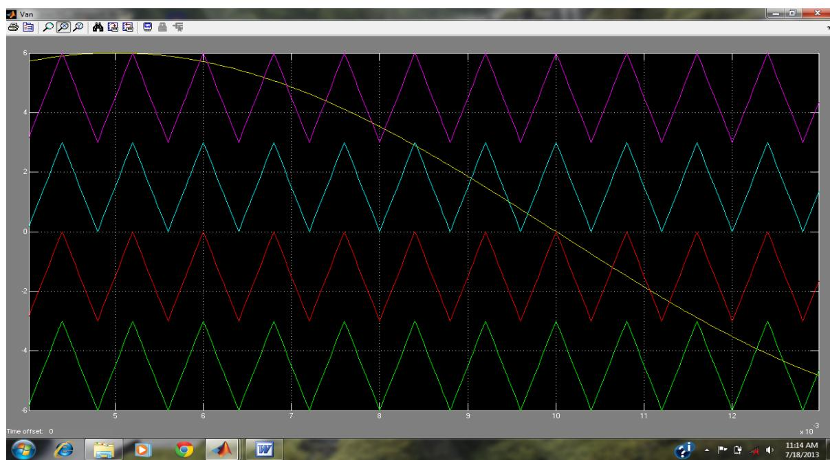
Fig.2 Triangular Waveform Simulation of Five Level Diode Clamped Inverter (PD PWM Technique)
